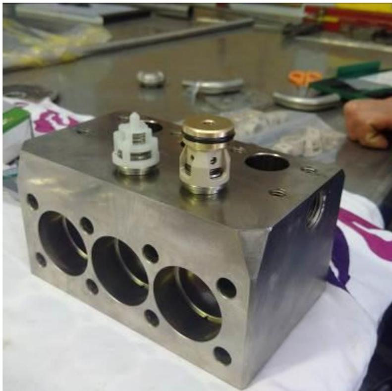
*New valve cages (left) were wearing out far too quickly. New high-performance valve cages (right) suggested by Cut To Size Plastics were a welcomed solution*
